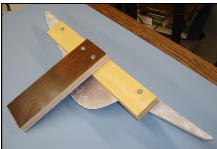
Mounting holes have been marked on a piece of scrap wood, which will be used to temporarily mount the hull so the deck can be planked. This template will also be used to determine the final location for the mounting holes on the finished backboard.
